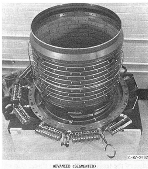
Fig. 25 Conventional and segmented combustor liners instrumented for testing
